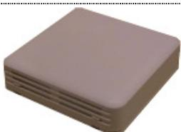
The **room temperature sensor** is suitable for wall fastening. The wiring is made with use of a shielded cable like for the duct sensor. Also in this case the polarity does not affect the measurement precision. The use of a room temperature sensor is precondition for the function of the backup mode and ventilation at night.
