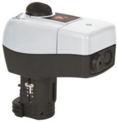
A robust construction was chosen for the Rosenberg- **valve-drive motor** Type AME 435. The servo drive also provides the option of an emergency manual operation. In this case the valve must be adjusted with a control knob installed outside the house. The raw percentage opening of the valve can be read on a scale at any time. To ensure a correct function the DIP switches attached to the gear must be set as follows:
