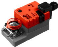
The **Bypass flap- servo motor** is pre-assembled in the SupraBox COMFORT and finally wired. The damper servo motor used for the bypass flaps has no limit switch and an overload protection. If the end position of the flap or the motor is reached they stop automatically.
