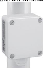
If a return temperature control is applied, the use of a **contact sensor** is necessary. This must be fixed at the return of the hot water coil in the same way as the contact thermostat. The wiring to the switch cabinet should be made with use of a shielded cable (J-Y (St) Y 4x 0, 6). The polarity of the connections at the control box and at the contact sensor does not affect the function.
